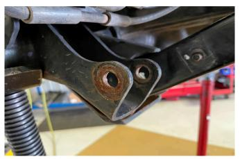
Carefully lower the axle approximately 2 inches, making sure that no other components are binding or stretched.
